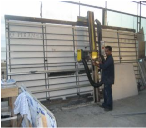
Cladding Cutting Machine
