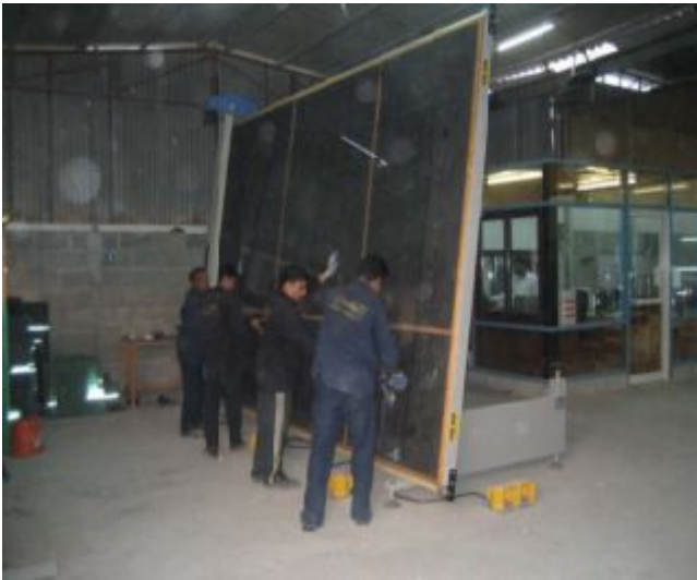
Loading Glass Table Cutting
